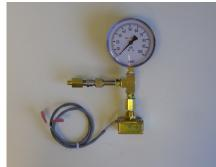
Complete assembly of pressure/vacuum switch, 4" diameter pressure/vacuum gauge, and gas specific DISS union demand check valve. Entire assembly is cleaned for oxygen service.
