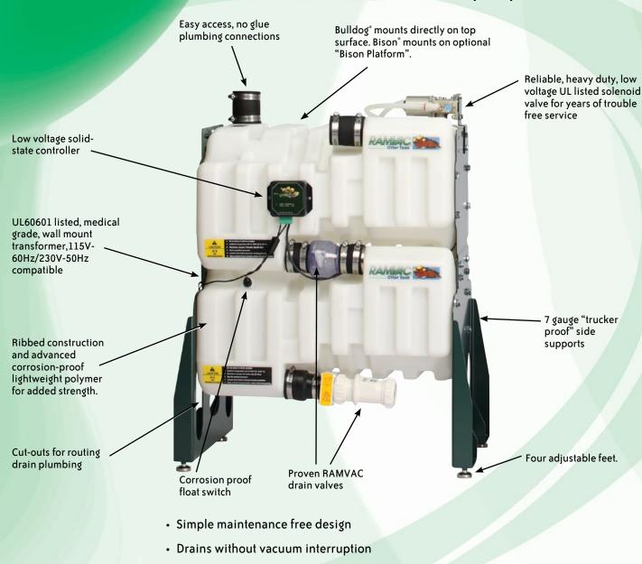
· Significantly reduces the size and number of separating tanks
